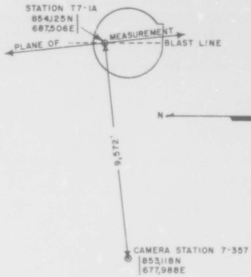
Figure 3.16 Shot 6, Plane of Measurement for Direct Shock Photography Films 28081 and 28084.
